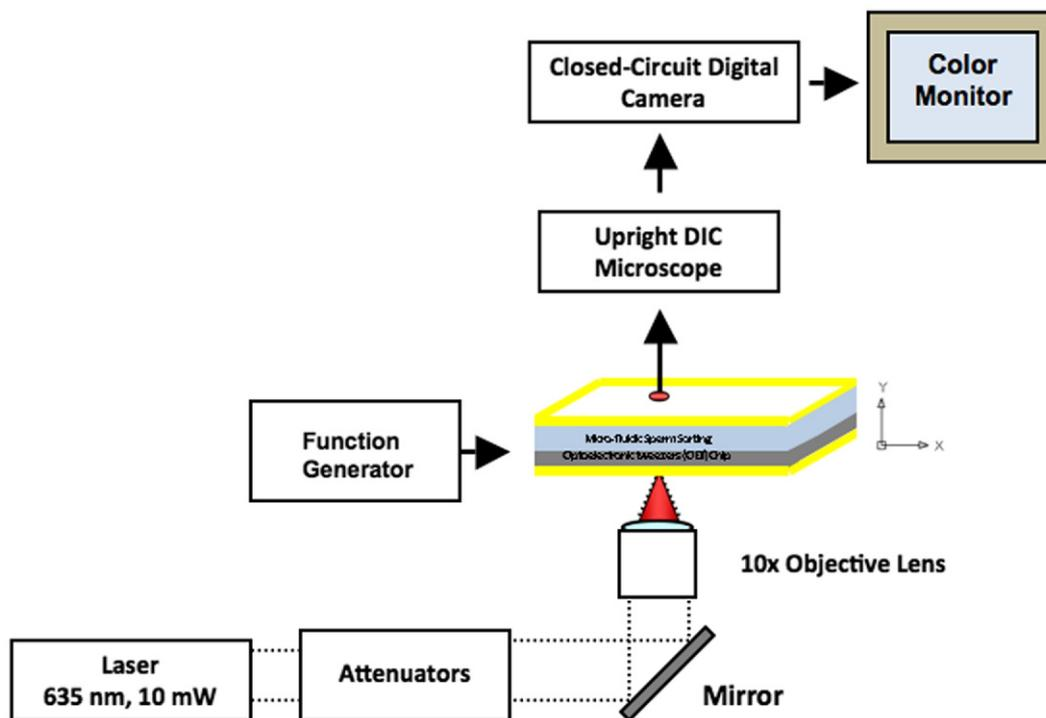
**Figure 3.** Primary OET sperm sorting platform components include micro-fluidic sperm sorting chamber in slide chip (*Function Generator*) mounted on movable stage of differential interference contrast microscope. Laser energy/light is projected on sperm sorting micro-chamber (chip) from beneath stage. Digital camera connected to microscope captures image and displays it on color monitor.
