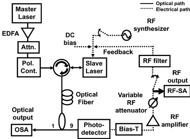
Fig. 2. Experimental setup for measuring RF modulation and feedback properties of an OIL-OEO. EDFA: erbium-doped fiber amplifier; Attn.: optical attenuator; Pol. cont.: polarization controller; OSA: optical spectrum analyzer; RF-SA: RF-spectrum analyzer.
