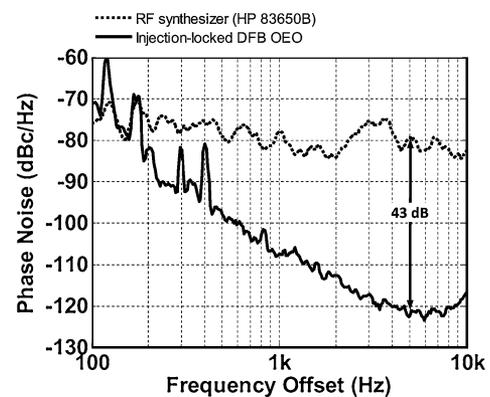
Fig. 11. Measured phase noise of an OIL-OEO-generated RF signal centered at 20 GHz using a DFB as the slave laser. 43-dB improvement occurs at frequency offset of 5 kHz, compared to the HP 83650B RF synthesizer.
