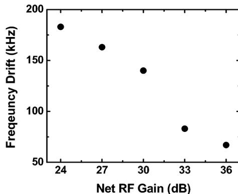
Fig. 9. Measured frequency drift of OIL-OEO signal as a function of RF gain of the link. RF gain is adjusted by an RF attenuator. The frequency drift is measured over a 30-s window.
