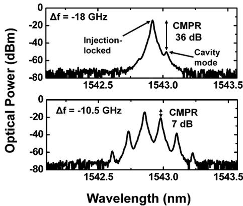
Fig. 4. Optical spectra of open-loop system without RF modulation for  $\Delta f = -18$  GHz (top) and  $\Delta f = -10.5$  GHz (bottom). CMPR is 36 and 7 dB, respectively.
