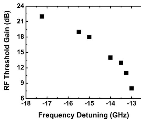
Fig. 8. RF threshold gain as a function of frequency detuning. The lowest threshold gain of 7 dB is achieved at  $\Delta f = -13$  GHz.
