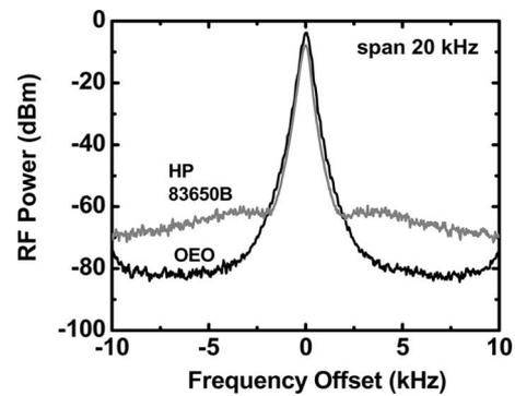
Fig. 10. Measured RF spectrum of an OIL-OEO-generated RF signal with a 17-km fiber loop employed. The OIL-OEO RF signal is generated at 20 GHz, and is compared with a 20-GHz RF signal directly from an HP 83650B synthesizer.
