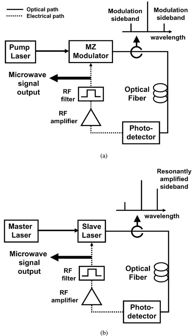
Fig. 1. Schematic of (a) standard OEO and (b) OEO using OIL semiconductor lasers. Optical spectrum of OIL OEO exhibits a significant enhancement of the longer wavelength modulation sideband due to the cavity resonance amplification in the injection-locked lasers.
