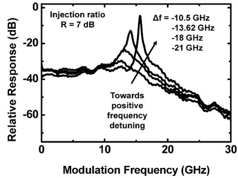
Fig. 3. Measured frequency responses of the open-loop system shown in Fig. 2. Narrow-band enhancement is achieved when the frequency detuning is close to the positive edge of the locking range.
