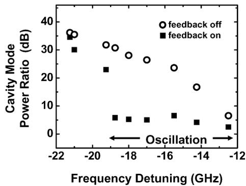
Fig. 7. CMPR versus frequency detuning with (open circle) and without (solid square) optoelectronic feedback. The loop starts to oscillate at  $\Delta f = -18.7$  GHz.
