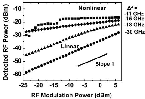
Fig. 5. RF output power versus RF modulation power for various frequency detuning values. Corresponding CMPRs are 6.3 dB ( $\Delta f = -11$  GHz), 19 dB ( $\Delta f = -15$  GHz), 36 dB ( $\Delta f = -18$  GHz), and  $>50$  dB ( $\Delta f = -30$  GHz).
