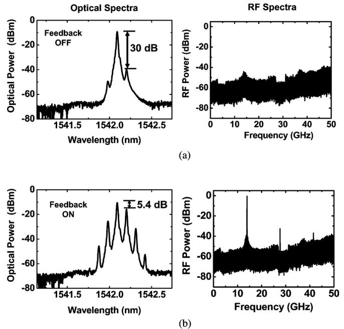
Fig. 6. Optical and RF spectra of OIL-OEO loop (a) without and (b) with feedback.  $R \sim 5$  dB,  $\Delta f = -18$  GHz. The feedback significantly enhances the modulation sidebands from loop oscillation.
