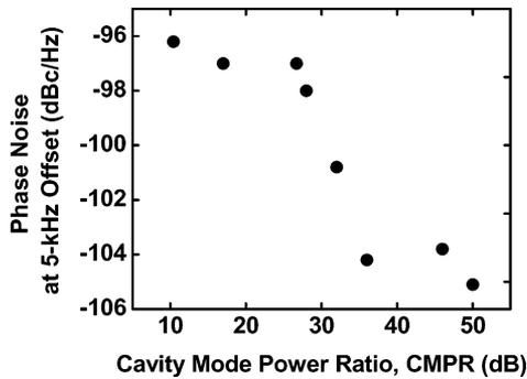
Fig. 12. Measured phase noise as a function of CMPR. Phase noise is measured at a frequency offset of 5 kHz at a center frequency of 20 GHz.
