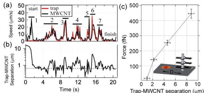
FIG. 2. (Color online) (a) Absolute speed and (b) absolute separation of MWCNT and laser during the course of the trapping measurement in Fig. 1. (c) Trapping stiffness measurement from force on MWCNT measured from Stokes drag exerted by the trapping laser during trace 1 in Fig. 1. Inset: schematic of fluid flow around MWCNT.
