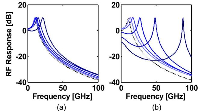
Fig. 3. (Color online) Frequency responses for two different lasers: (a)  $Q=13,320$ , (b)  $Q=3330$ . The curves in each set are the maximum resonance frequency at a given injection ratio. Light to dark curves correspond to  $R_{ext} = -10, -5, 0, 5, \text{ and } 10 \text{ dB}$ , respectively. Dotted curves correspond to the free-running response.
