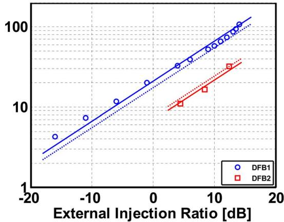
Fig. 4. (Color online) Comparison of theory with experimental data for maximum resonance frequency enhancement. The points are sets of  $\Delta\omega_{R,max}$  at different injection ratios, for two different lasers. Solid lines, fits of Eq. (11); dotted lines, calculated  $\Delta\omega_{R,max}$  based on DFB stop-band width.
