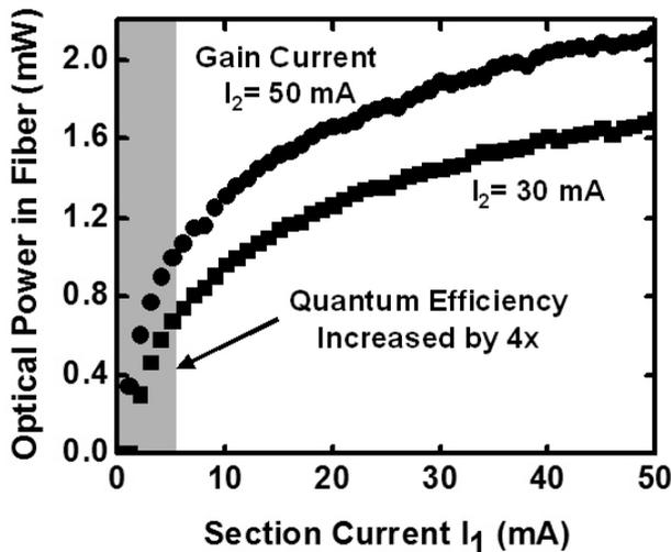
FIG. 4. Measured optical power versus the bias current on section showing the effect of gain-lever modulation.
