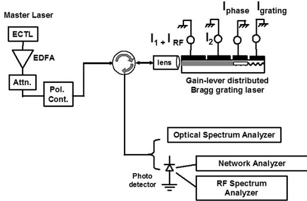
FIG. 3. Experimental setup for measuring RF performance of a gain-lever DBR laser with and without injection locking. (ECTL: external cavity tunable laser; EDFA: Erbium-doped fiber amplifier; Attn.: optical attenuator; Pol. cont.: polarization controller).
