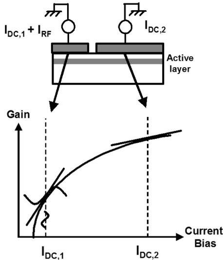
FIG. 1. Gain-lever effect in semiconductor lasers, after [3].
