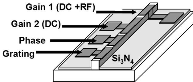
FIG. 2. Schematic of distributed Bragg reflector (DBR) laser for gain-lever modulation.
