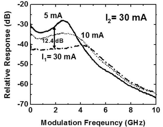
FIG. 5. Measured modulation responses of the gain-lever DBR laser for various operating conditions.
