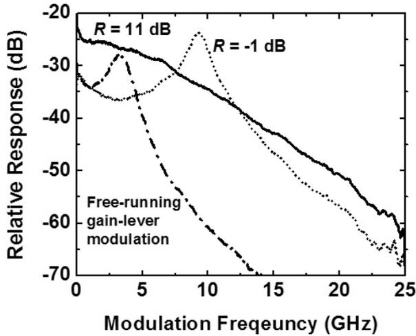
FIG. 7. Measured frequency responses of a free-running, strong ( $R=-1$  dB,  $\Delta f=-7.4$  GHz), and ultra-strong ( $R=11$  dB,  $\Delta f=-32$  GHz) injection-locked DBR laser with gain-lever modulation.
