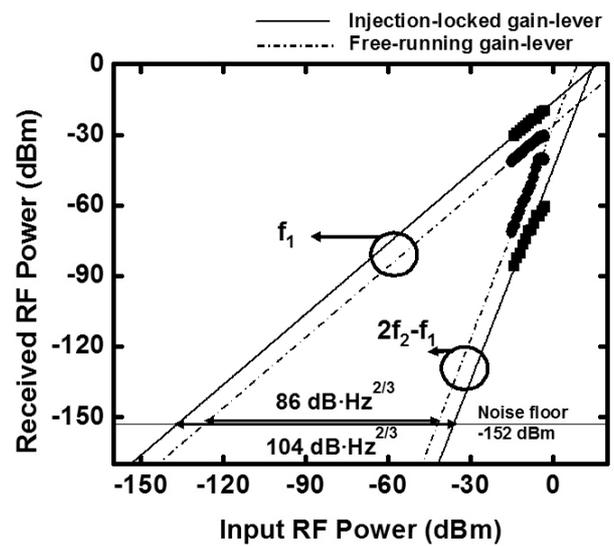
FIG. 10. Measured SFDR of the link with a directly modulated gain-lever DBR laser ( $f_1=2.0$  GHz,  $f_2=2.1$  GHz).
