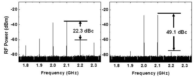
FIG. 9. Measured RF spectra showing the two-tone intermodulation distortions ( $f_1=2.0$  GHz,  $f_2=2.1$  GHz) of the gain-lever DBR laser under (a) free-running and (b) ultra strong injection-locking conditions ( $R=11$  dB,  $\Delta f=32$  GHz).
