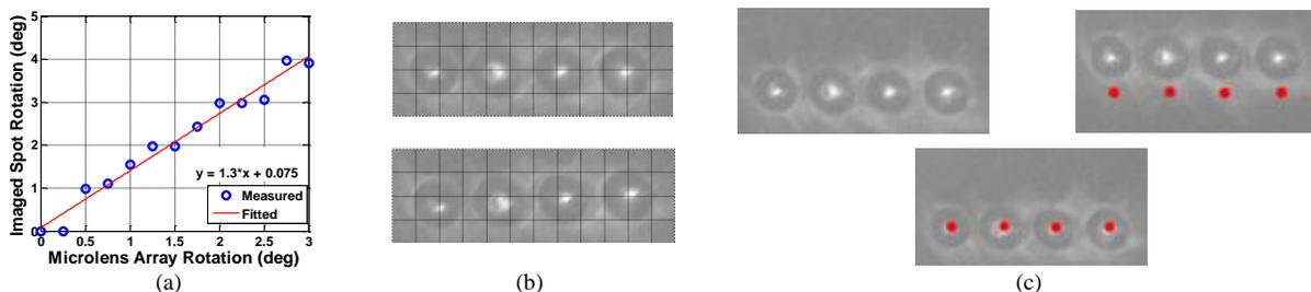
Fig. 4. Active alignment measurements. (a) The measured image rotation as a function of the microlens array rotation. (b) (*top*) Spot image at 0° rotation. (*bottom*) Spot image at 3° rotation. (c) (*top left*) Beam spot location at 0° board tilt. (*top right*) Beam spot location at 0.7° board tilt. Spots are displaced by 157.4  $\mu\text{m}$  from the original positions (red spots). (*bottom*) Spots are moved back to 0° location with the millimeter lens displaced by 170  $\mu\text{m}$ .
