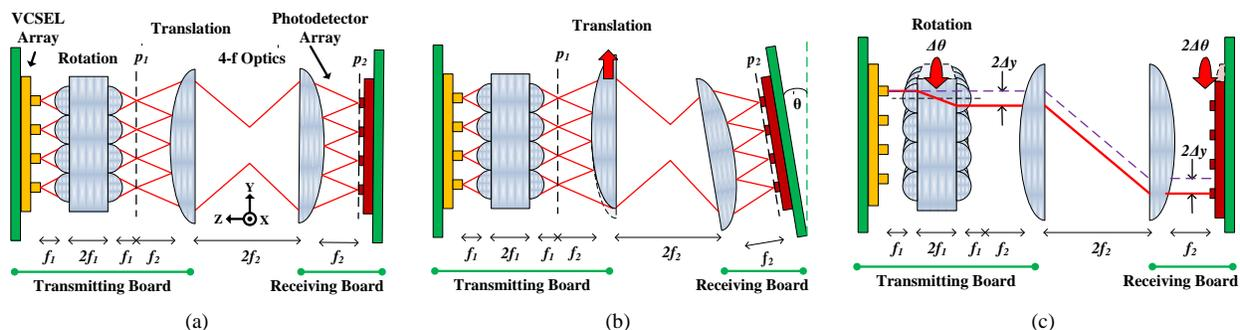
Fig. 1 Illustrations of a proposed free-space board-to-board optical interconnect system integrated with MEMS actuators. (a) shows the full diagram at perfect alignment. (b) shows a board tilt away from the Y-axis being corrected with our translational MEMS lens scanner. (c) shows a board rotation about the Z-axis (optical axis) being corrected with our MEMS rotation stage.
