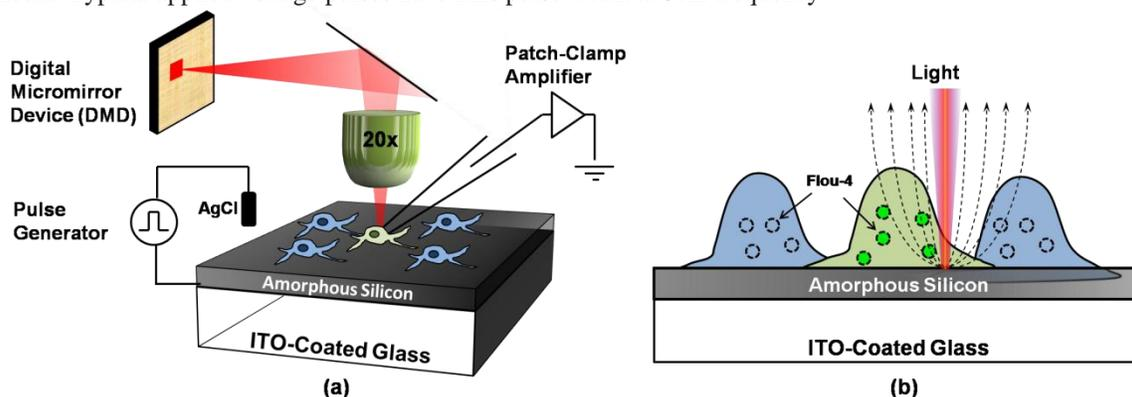
**Fig 1. (a) Schematics of the optical neural stimulation setup.** DMD provides dynamic light addressing capability. The open top design allow patch-clamp recording. **(b) Schematics of device operation.** Light induces local electric field, which depolarize the nearby neurons. The depolarization causes increase of  $\text{Ca}^{2+}$  in the cell, and the event can be monitored by Flou-4 fluorescent intensity increase.
