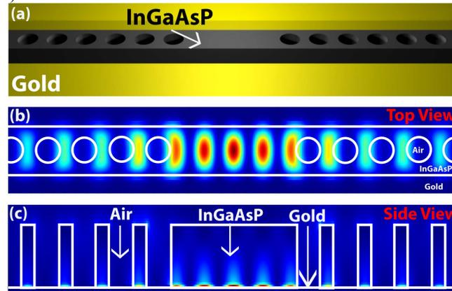
Fig. 1: (a) A schematic of the device, (b) the top view and (c) the side view of the fundamental mode is shown. The color scale represents electric field intensity. The mode volume is significantly reduced due to the surface nature of the plasmonic mode. The crystal structure is outlined in white lines, and the materials are labeled accordingly.
