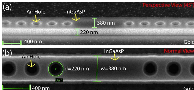
Fig. 2: Scanning electron micrographs of (a) a perspective view and (b) a surface normal view of the final fabricated structure are shown. The final device dimensions are noted along with scale bars. A semiconductor layer is patterned on a gold film.
