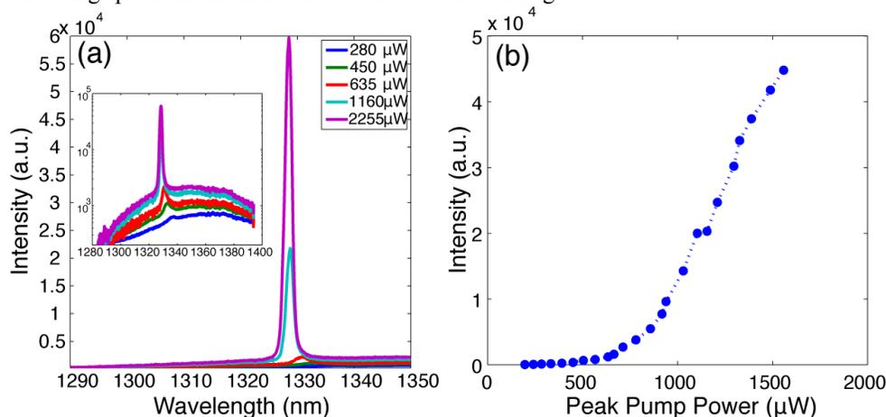
Fig. 3: (a) Power dependent lasing spectrum (inset: log-scale) and (b) L-L curve a characteristic laser is shown. A soft threshold is observed as expected from nanocavity lasers. The clamping of spontaneous emission strongly suggests light evolution by stimulated emission.
