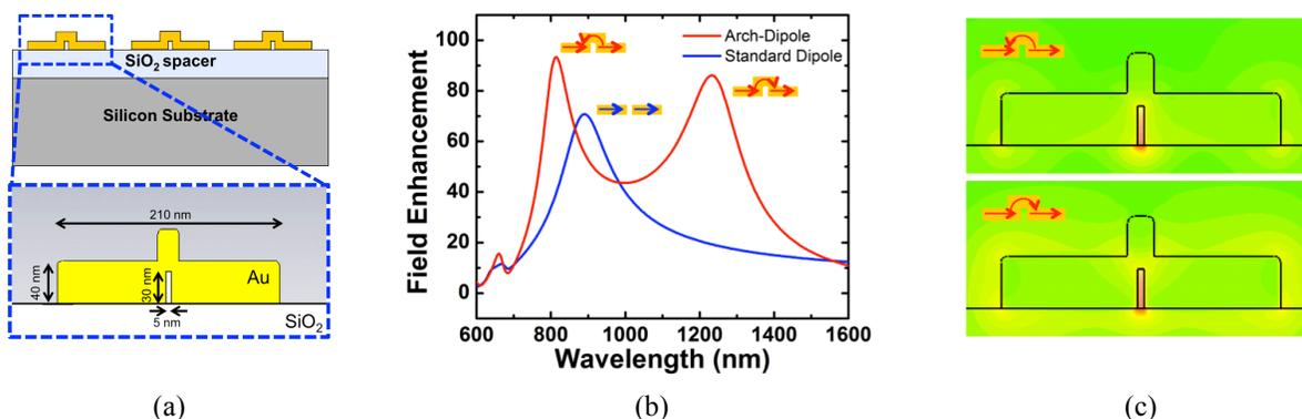
Fig. 1 (a) Schematic of the arch dipole antennas. The dimensions of the antenna is shown in the inset. (b) E-field enhancement simulation. The field is measured at the center of the gap. The current distribution of the antenna is shown next to each resonance peak. (c) E-field distribution of two arch-dipole antenna modes.
