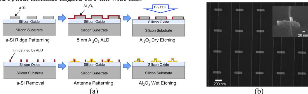
Fig. 2 (a) Fabrication process. (b) SEM images of optical antenna array aligned on 5 nm fins. Inset shows perspective view of a single antenna.
