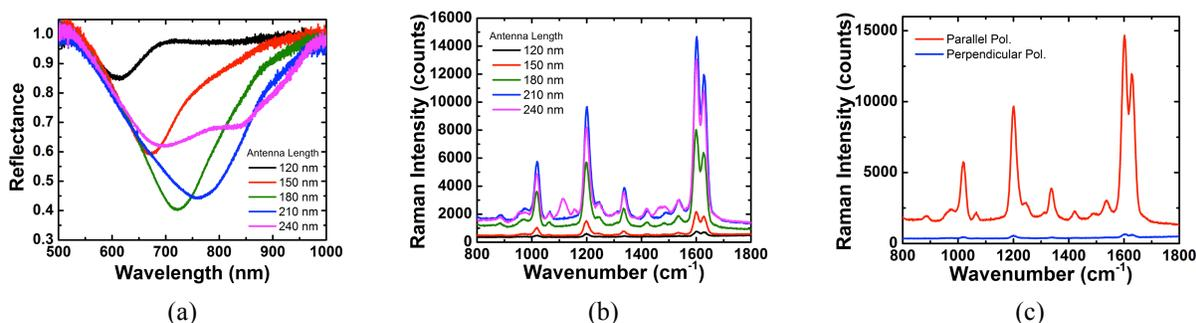
Fig. 3 (a) Reflectance measurement of fabricated optical antenna arrays with antenna length variations. (b) Measured BPE SERS spectra. (c) SERS comparison with two different excitation polarizations.
