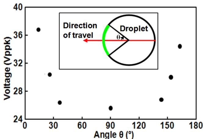
Fig. 2: Bias voltage required to move droplet at  $3\text{mm}/\text{s}$  versus angle  $\theta$  subtended by the ring electrode (see inset). Minimum voltage (strongest actuation) is obtained at  $\theta = 90^{\circ}$ . Effective actuation of droplets is achieved with angles as small as  $\theta = 45^{\circ}$ .
