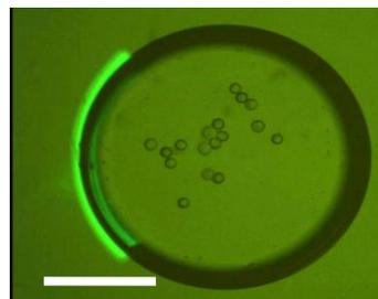
Fig. 3b: Quarter-ring-shaped light pattern projected on a droplet. Hydrogel microspheres are contained within the droplet. Temperature increase of 0.35°C is observed. The scale bar is 1mm.
