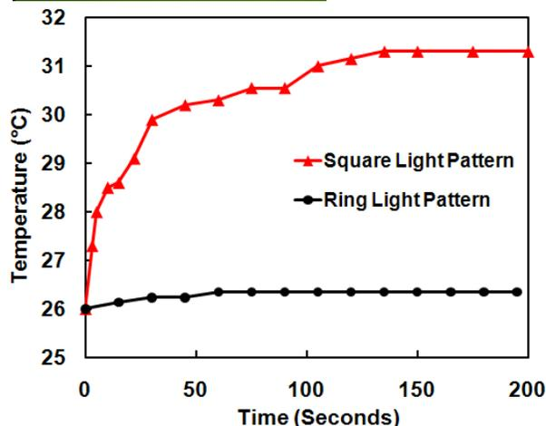
Fig. 4b: Temperature within droplet against time, for both the illuminated side of square-shaped electrode and the quarter-ring-shaped electrode.
