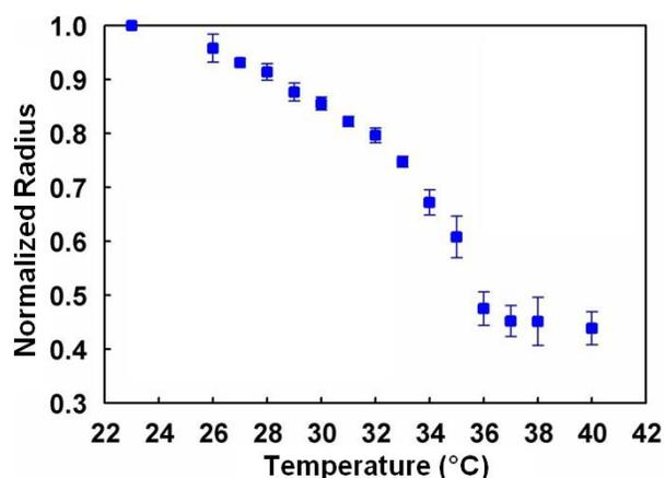
Fig. 4a: Calibration curve used to derive droplet temperature in-situ, as a function of measured hydrogel microsphere radius, as presented in [3].
