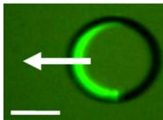
Fig. 1b:  $2\mu\text{l}$  droplet actuated in the direction of arrow using half-ring electrode. Speed  $3\text{ mm}/\text{s}$ , voltage  $25.6\text{ Vppk}$ , frequency  $10\text{ kHz}$ , scale bar  $1\text{mm}$ .
