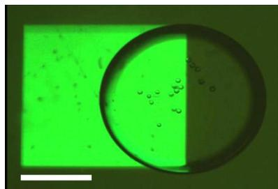
Fig. 3a: Square-shaped light pattern projected on a droplet. Hydrogel microspheres are contained within the droplet. Temperature increase of 5.3°C is observed. The scale bar is 1mm.
