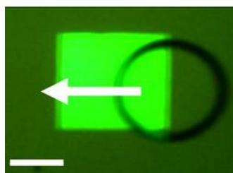
Fig. 1a:  $2\mu\text{l}$  droplet actuated in the direction of arrow using square electrode. Speed  $3\text{ mm}/\text{s}$ , voltage  $24.8\text{ Vppk}$ , frequency  $10\text{ kHz}$ , scale bar  $1\text{mm}$ .
