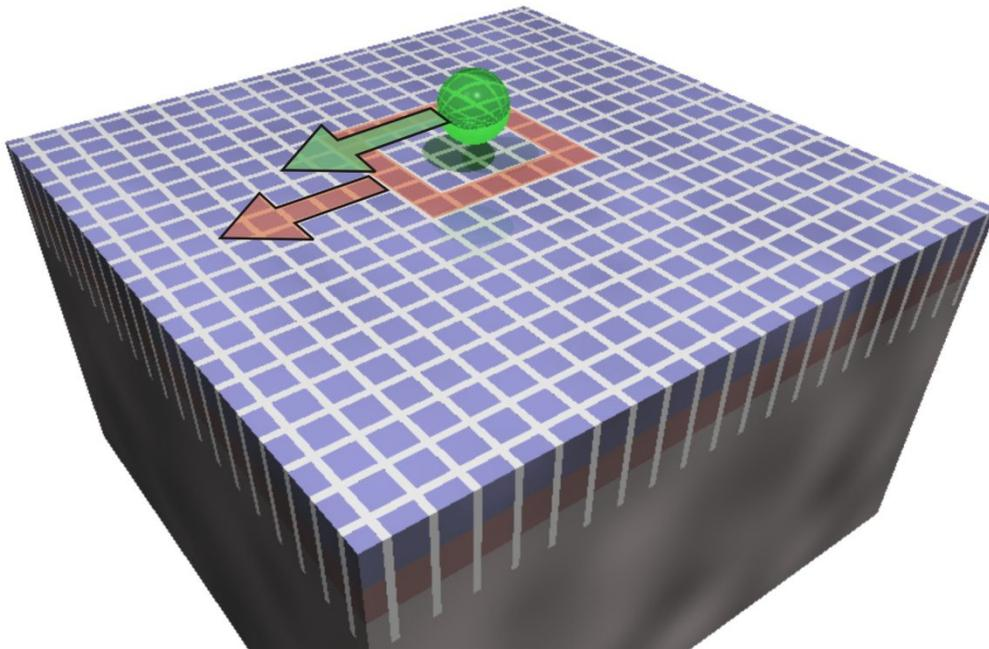
Fig. 1. A Ph-OET device is shown consisting of two layers of doped silicon which is etched into the pixilated pattern. The device can be illuminated with a square ring of light surrounding the cell to be trapped. The ring can then be moved causing the cell to move as indicated by the arrows.
