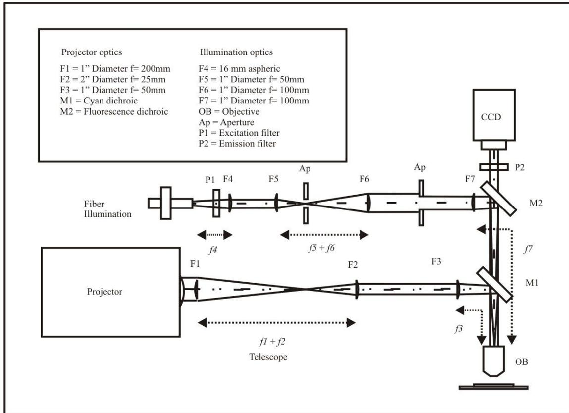
Fig. 5. The optical setup used for the Ph-OET experiments is a microscope as shown here. The optical pattern generated by a data projector is focused onto the chip through a 20x objective. The chip is also illuminated by a fiber illuminator which excites the fluorescence from the cells.
