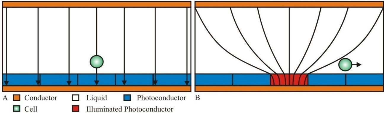
Fig. 2. A) An AC voltage is placed across the two conductive layers producing an electrical field as indicated by the electrical field lines (arrows). B) When a small area is illuminated the electrical field is concentrated in this area producing an electrical field gradient which causes the repulsion of the particle.
