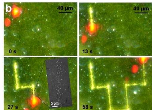
Fig. 3. Real-time patterning of gold nanoparticles (mixture of  $60 \text{ nm}$  and  $90 \text{ nm}$  in diameter) using a manually controlled laser spot. The field gradients formed in the vicinity of the optically defined virtual electrodes interact with
