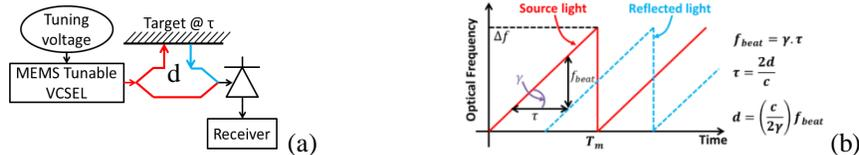
Figure 1. Linear FMCW LIDAR principle of operation. a) System block diagram; b) Graphic representation.
