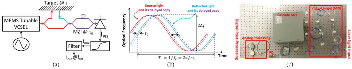
Figure 2. Proposed system operation. a) Architecture; b) Graphic representation; c) Measurement setup.
