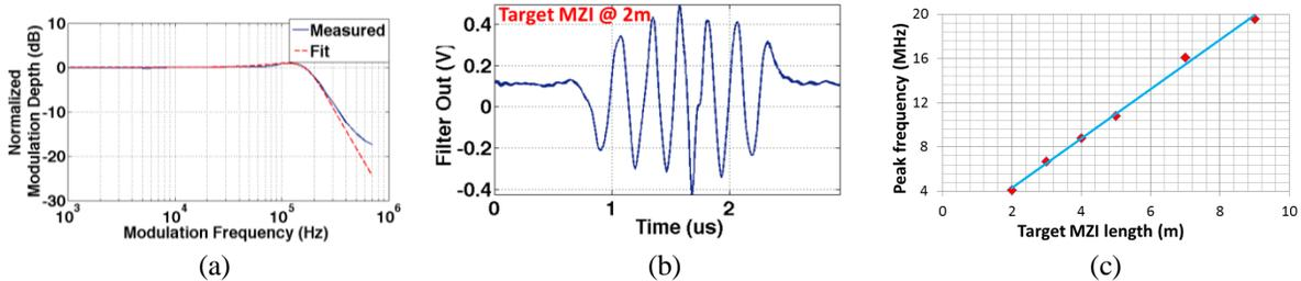
Figure 3. Measurement Results. a) Tuning frequency response; b) Filter output in Fig. 2a; c) Peak beat frequency versus MZI length.
